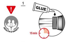
Before you apply the heating element, spread the Loctite glue (included in the set) on the middle of the thread circumference.
