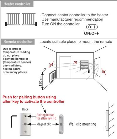
START: Heater controller and remote controller pairing
