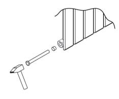
\* Diverter should be installed into the flow side of the radiator
