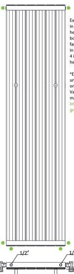
Except 500 & 600mm heights, in 800, 1000, 1200, 1400 & 1800mm heights there are \*6 inlets. The bottom 2 inlets are under the far left and right profiles. in 500 & 600mm heights there are 4 inlets, none under the bottom header.
