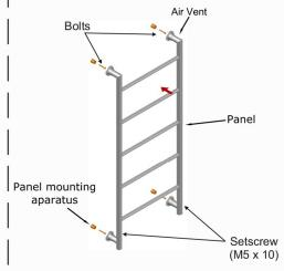
Fix the panel mounting apparatus to
