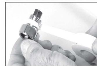
Wrap PTFE tape clockwise around the tail thread
