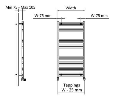
Tapping from wall: 75-105 mm. Radiator front to wall 85-115 mm.
