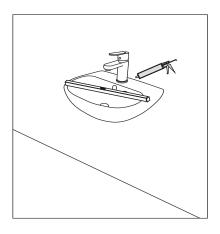
3) Take away the basin, use Ø10mm driller to make two 60mm depth holes following the marks.
