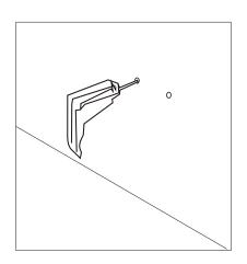
2) Someone holds the bsain on its place, the other one remove the pedestal away, then put marks on the wall for the installing holes (two).
