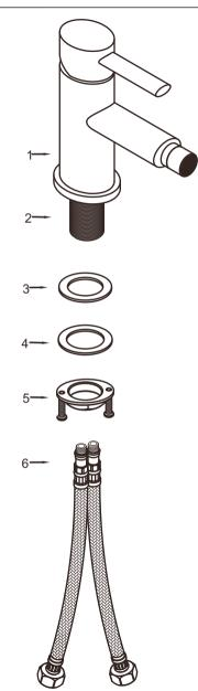
56.2041 Cortauld mono bidet c/w clicker waste Manufacturers Code: 50314 **COMPONENTS** The monobasin contents the following: 1 Single lever bidet mixer 2 Connection sleeve with male screw 3 Rubber sleeve gasket 4 Steel sleeve gasket 5 Oval fixing nut 6 Flexible hose 7 Pop-up waste 8 Upper washer 9 Under washer 10 Fixing gasket 11 Fixing nut check that all parts are correct
