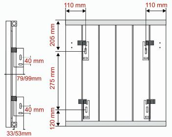
\*600mm height radiators have one hanger fixing position located 150mm from the top of the radiator.
