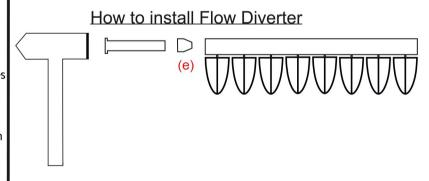
\*Diverter should be installed into the flowside of the radiator.
