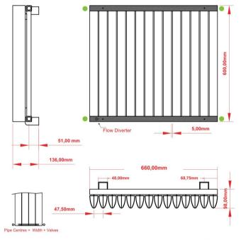
In total there are 4 inlets in 600mm. Height sizes. All 4 inlets are marked with green dots above.
