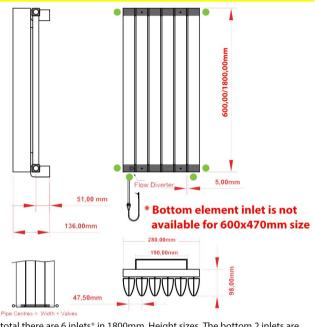
In total there are 6 inlets  $^{\ast}$  in 1800mm. Height sizes. The bottom 2 inlets are under the far left and right profiles.
