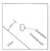
3) Drill a Ø 9mm hole accordingly.
