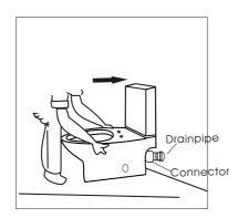
7) Fix and tighten the screw, cover the screw cap.
