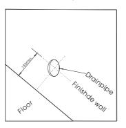
3) Drill a Ø 9mm hole accordingly.
