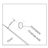
3) Drill a Ø 9mm hole accordingly.
