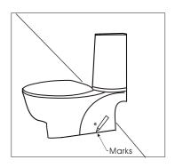
4) Put the swelling gasket into the hole and fix the plastic holder with screw.
