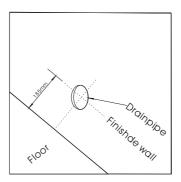
3) Drill a Ø 9mm hole accordingly.
