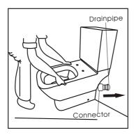
7) Fix and tighten the screw, cover the screw cap.
