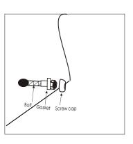
8) Connect the inlet valve with soft pipe and multivalve.
