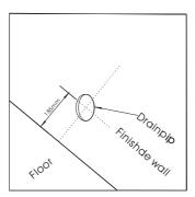
3) Drill a Ø 9mm hole accordingly.
