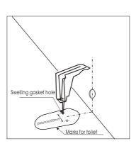
2) Marks round the toilet on the floor, and figure out the screw hole.
