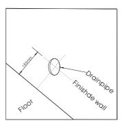
3) Drill a Ø 9mm hole accordingly.
