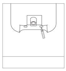
4) Put the expanding plastic into the hole, then fix the bolt with 60mm out of the hole.
