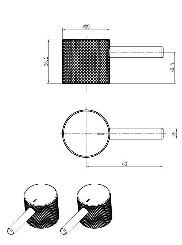
FULL knurling brass PAIR handle with round lever for body two holes tap
