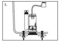
Unlock the Fixing Clip to adjust the Overflow Pipe to desired height, then lock the Fixing Clip.
