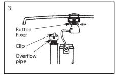
Fix Clip on the Overflow Pipe.
