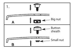
Turn the Nut and loosen it. Install the Button on the Tank Lid and fix the Nut properly. Installation A for Ø4cm hole in the Tank Lid. Installation B for Ø2-Ø3cm hole in the Tank Lid.
