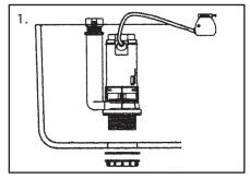
Disassemble Lock Nut, Plastic Washer for VALVE installation. Position the VALVE inside tank. Push down on the Valve Body while attaching Plastic Washer and tightening Lock Nut.
