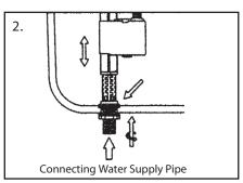
Position VALVE inside tank. Push down on the Valve Shank (not the top) while tightening Lock Nut. Screw the Valve Shank clockwise and pull the Valve Body to the correct height.
