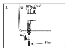
Adjusting the water level by screwing Float Bolt and move the Float Housing up or down along the Valve Body to join with the Float. The Float Housing should be attached to the Float and the Arm isn't raised. Take out the Filter and clean it often.
