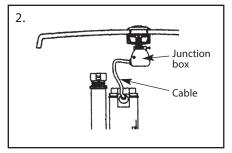
Make the Cable smooth, install the Button on the Junction Box and then close the Tank Lid. Fill the Tank with water and push the Full&Half Button to check whether the flushing is normal or not.
