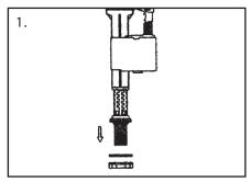
Disassemble the Lock Nut for valve installation.
