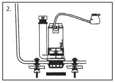
Nest the Tank To Bowl Washer in the Lock Nut and position the TANK on the Toilet Bowl properly. Disassemble the Tank To Bowl Bolts. Fix the Tank to Toilet Bowl the Tank To Bowl Bolts tightly.
