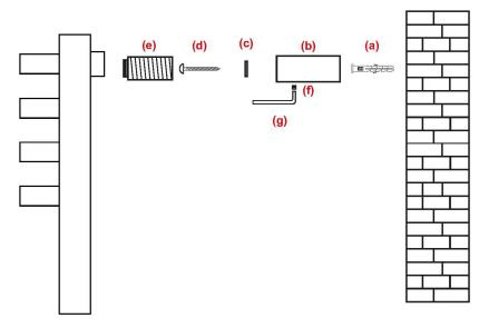
Maximum working pressure of this radiator is 4 bar. This radiator is to be used on Domestic Central Heatting. systems only. (Not suitable for use on direct hot water systems).
