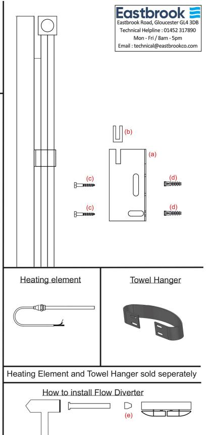
\*Diverter should be installed into the flowside of the radiator.
