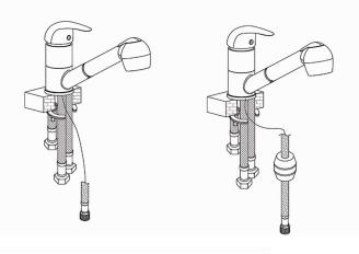
6. Insert the shower hose into the tap and connect the hose to
