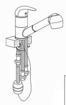
2. Install the inlet pipes and outlet pipe to the tap
