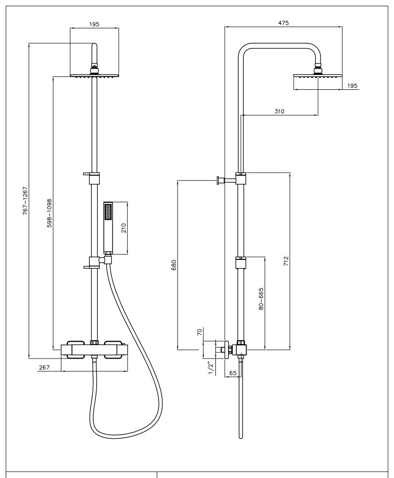
Square Wall Mounted thermostatic valve with rigid riser, fixed head and shower kit AB4191 v1
