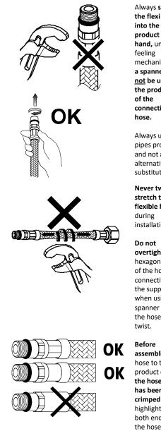
Always screw the flexi hoses product only by hand, until mechanical rest, a spanner must not be used on the product end connecting
