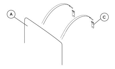
9. If required adjust the brackets to make sure the mirror is level.
