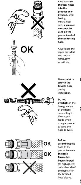
The braiding on the flexible hose must not be in contact with anything else, for example chemicals, internal or external room walls or dissimilar metals or materials or sharp objects. Hoses must not be double bent in multiple directions kinked or looped. Observe the minimum bend radius of 50mm. 50mmØ
