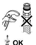
the flexi hoses into the product only by hand, until feeling mechanical rest, a spanner must not be used on the product end of the connecting hose.
