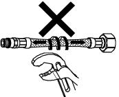
Never twist or stretch the flexible hose during installation.
