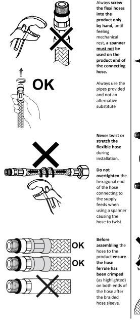
The braiding on the flexible hose must not be in contact with anything else, for example chemicals, internal or external room walls or dissimilar metals or materials or sharp objects
