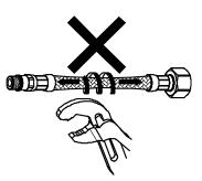
Never twist or stretch the flexible hose during installation.
