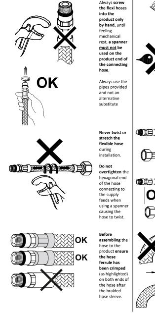
The braiding on the flexible hose must not be in contact with anything else, for example chemicals, internal or external room walls or dissimilar metals or sharp objects.
