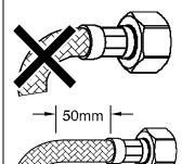
Both ends of the hose must have a minimum 50mm straight section before any bend.
