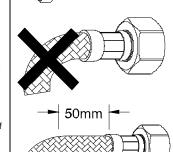
Both ends of the hose must have a minimum 50mm straight section before any bend.
