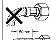
Both ends of the hose must have a minimum 50mm straight section before any bend.
