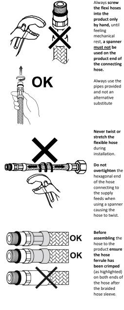
The braiding on the flexible hose must not be in contact with anything else, for example chemicals, internal or external room walls or dissimilar metals or materials or sharp objects.
