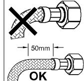
Both ends of the hose must have a minimum 50mm straight section before any bend.
