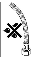
The braiding on the flexible hose must not be in contact with anything else, for example chemicals, internal or external room walls or dissimilar metals or materials or sharp objects.
