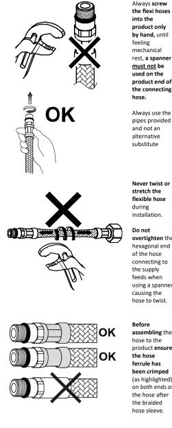
Always screw the flexi hoses product only by hand, until mechanical rest, a spanner must not be used on the product end of the connecting
