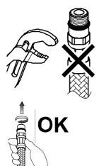
Always screw the flexi hoses into the product only by hand, until feeling mechanical rest, a spanner must not be used on the product end of the connecting hose.
