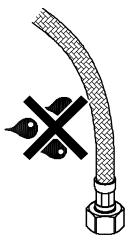
The braiding on the flexible hose must not be in contact with anything else, for example chemicals, internal or external room walls or dissimilar metals or materials or sharp objects.
