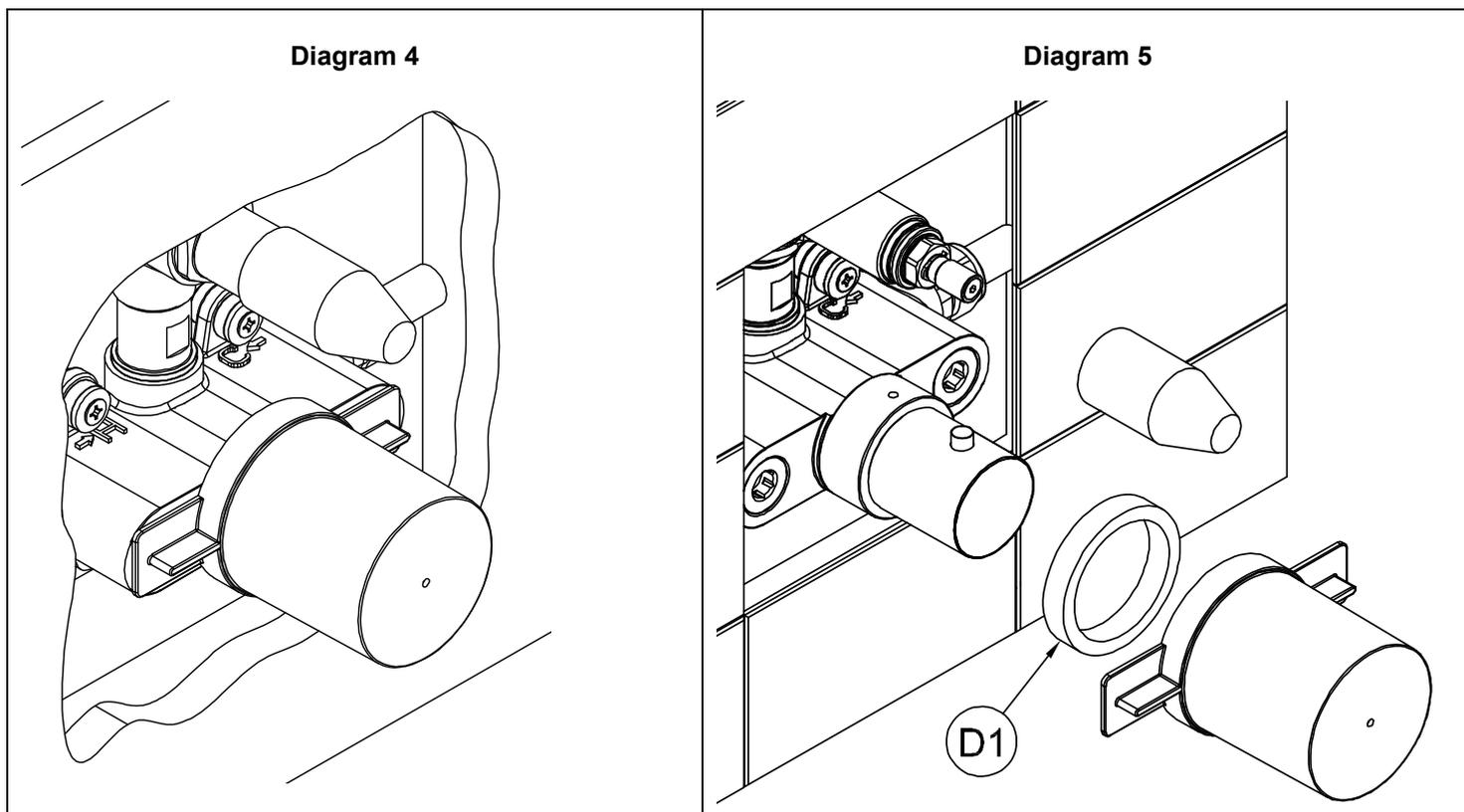
6. Make good the finished wall surface using tiles or similar, ensuring plastic valve caps (**C & D**) are in place as shown in **Diagram 4** to protect decorative parts. The tiles must overlap the finished shroud plate (**N**) by at least 15mm on each side of the plate. Do not tile over the inlet mesh filter ports (**A2**) and allow access to grub screw (**Y**).
