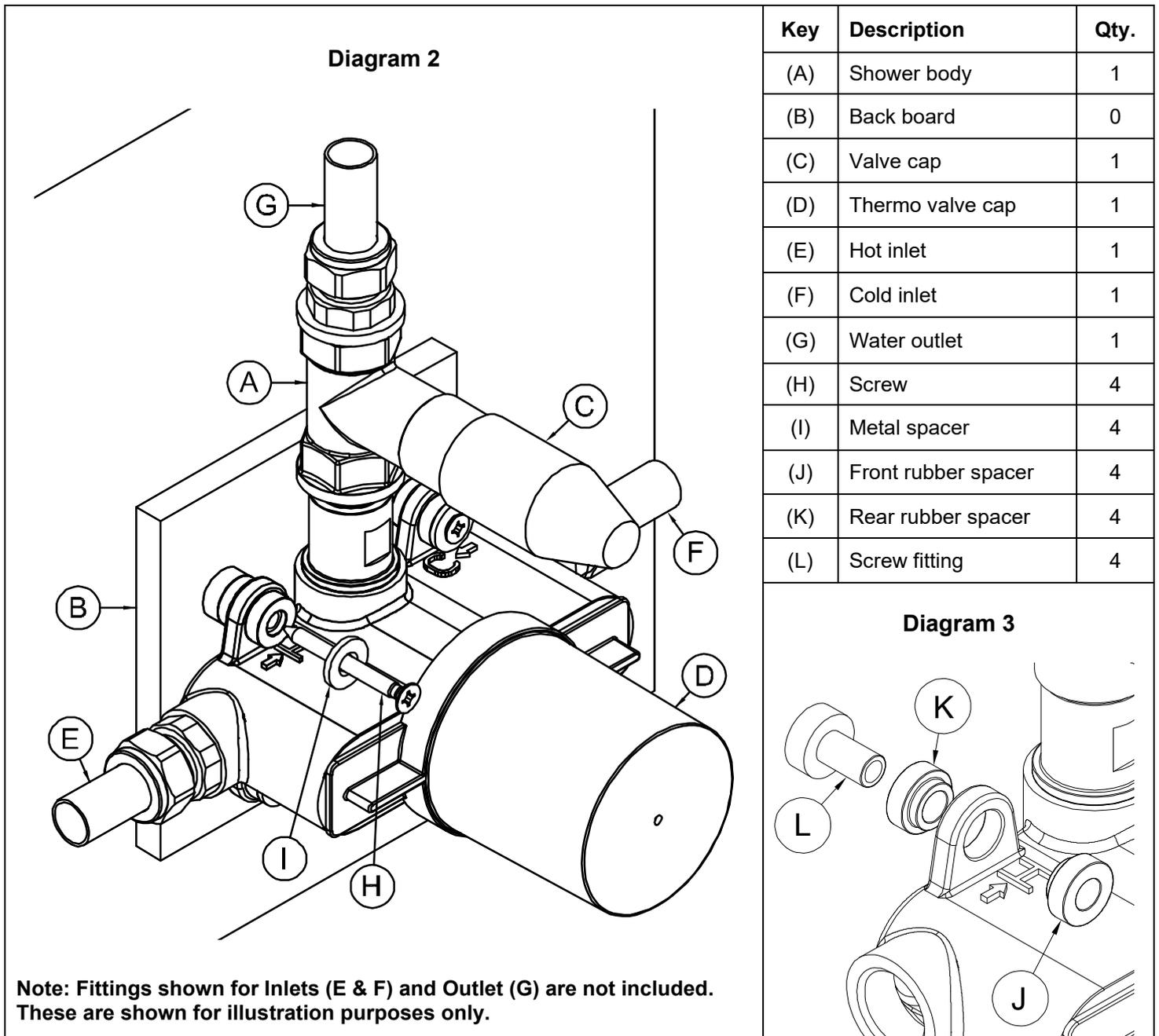
2. Fix inlet and outlet pipes securely to the wall using appropriate fixings. Inlet pipes should finish at the same height and be spaced as required.
