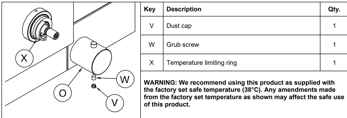
1. Note the alignment black pen marks already on the brass and plastic sections of valve body. Using a marker pen mark the current position onto the limiting ring (X) adjacent to the black mark on the brass and section of the valve.
