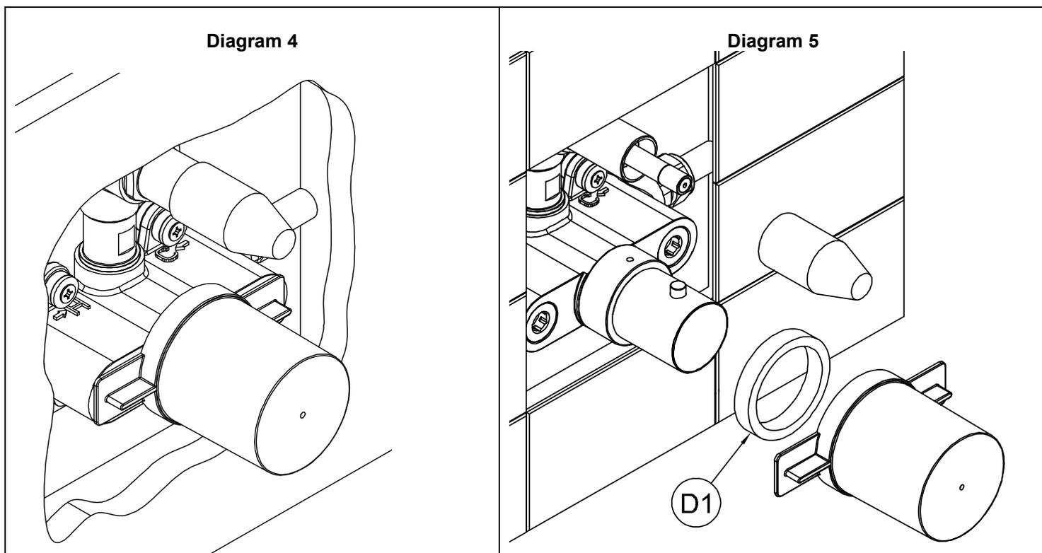
6. Make good the finished wall surface using tiles or similar, ensuring plastic valve caps (**C & D**) are in place as shown in **Diagram 4** to protect decorative parts. The tiles must overlap the finished shroud plate (**N**) by at least 15mm on each side of the plate. Do not tile over the inlet mesh filter ports (**A2**) and allow access to grub screw (**Y**).
