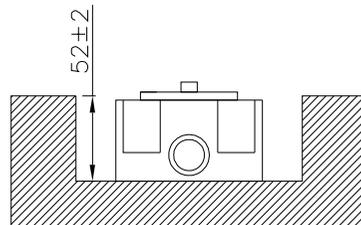
Create the seat for the body and for the supply pipes complying with the indicated sizes.
