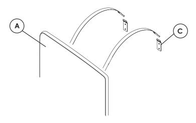
9. If required adjust the brackets to make sure the mirror is level.
