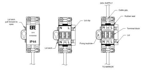
7.a Open the terminal box cover by gently pulling the lid latch forward, loosen the cable grip. 7.b Pierce the rubber seal, pass the wire through the seal, & cable grip, strip the wire to the required length.
