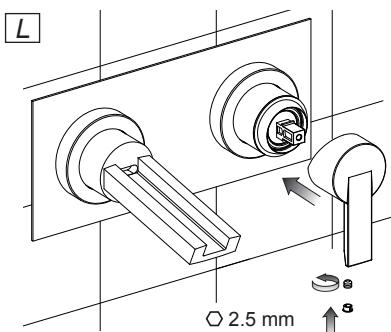
*Montaggio parti esterne in finiture diverse da CROMO - Installation of finished external parts different from CHROME.
