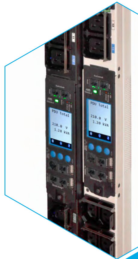
Figure 7: CPI Monitored Pro eConnect PDU has local and remote monitoring of power at the input, breakers and outlets. Measured values are presented on the LCD screen, through the PDU web GUI and can be shared with DCIM and other third-party monitoring software.
