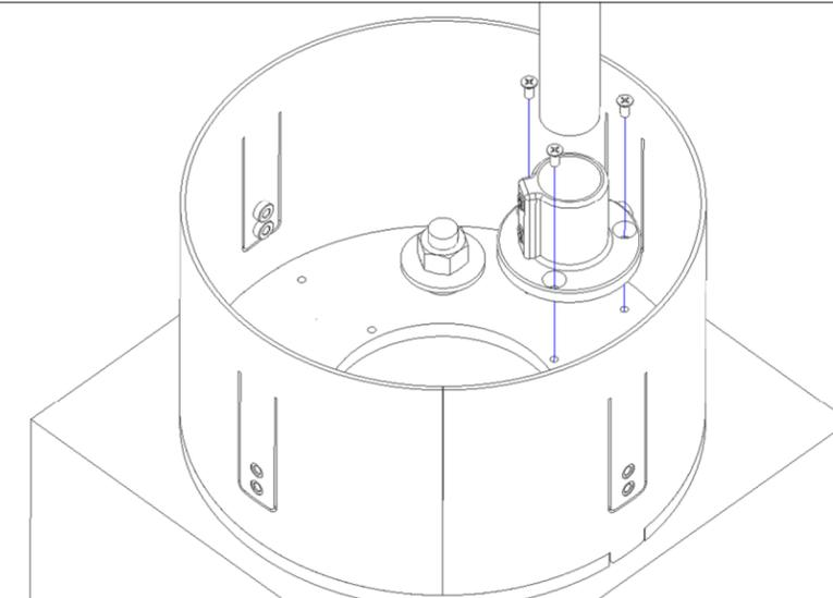
Fasten the Aluminum Pole Flange to the Anchor Base with the provided #8-32 Flat Head Screws. Slide the Fiberglass Pole into the Pole Flange and tighten the set screw.
