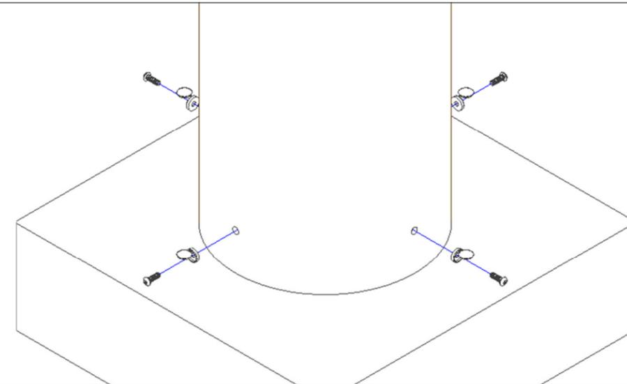
Place the Bollard over the equipment stand and fasten to the anchor base using the included 1/4"-20 tamper resistant screws and screw caps with the provided pin in hex bit. The bollard may be fastened to the lower set of holes on the anchor base to recess into the ground or cover excess hardware.
