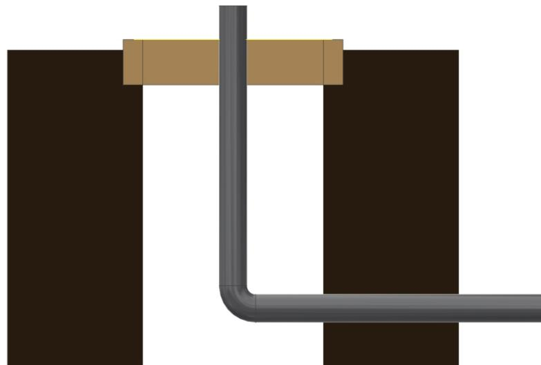
Dig the trench for laying conduit. Data and power cables must be separated when running conduit to the bollard. Place the conduit within the trench and up through where the anchor base concrete will be poured.
