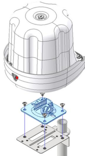
For the Aruba 270, 370, and 570 Series APs, fasten the R/A bracket to the Fiberglass Pole using the provided U-Bolts. Top of the R/A bracket using the included 1/4" - 20 Screws. The Fiberglass Pole may need to be trimmed. Once the access point is attached, plug in the cables.
