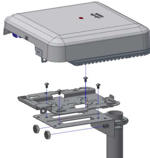
If mounting to the right-angle bracket, fasten the bracket to the Fiberglass Pole using the provided U-Bolts. Attach the Access Point to the T-Bar, or fasten the Cisco AIR-BRACKET using the included #8-32 Screws. The Fiberglass Pole may need to be trimmed. Once the access point is attached, plug in the cables.
