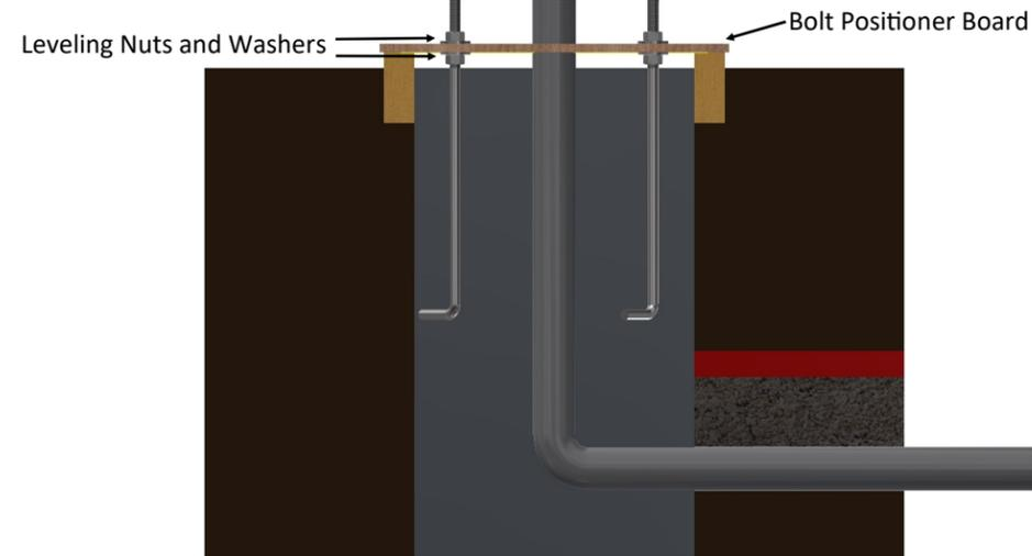
Press the anchor bolts into the wet concrete and vibrate to remove voids from around the anchor bolts and edges of forms. Level the bolt positioner board without pressing the bottom leveling nuts into the concrete. Cover and allow the concrete to set.
