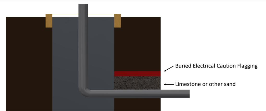
Follow local code requirements for buried conduit. Fill around the conduit with gravel if necessary. Mix and pour the concrete around the conduit. 3000 to 3500 psi concrete is recommended.
