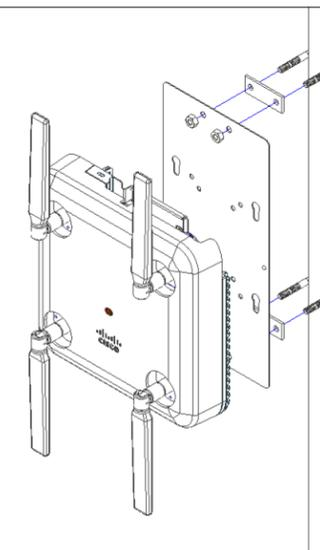
If mounting a Cisco Access Point, fasten the CCOAP Mounting Plate to the Fiberglass Pole using the provided U-Bolts. Attach the Access Point and plug in the cables.
