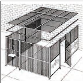
**Clear-Span Ceilings** – Clear-Span Ceilings provide additional security by enclosing the top of the Wire Cage Enclosures. Ceilings are constructed of the same material as the Modular Panels. Ceilings can be added to existing partitions without changing the layout. Ceilings attach to the top of the partition walls with a slotted angle. When required, support beams attach to the tops of posts. Note that ceilings are non-load bearing.
