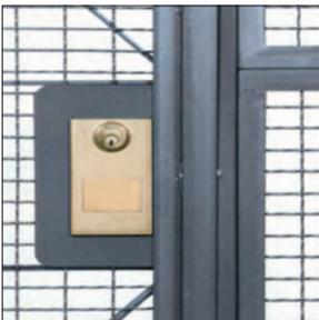
**Standard Door Locks** – The Standard Door Lock includes an exterior key actuated deadbolt with an internal recessed release latch. Standard locks are keyed differently unless keyed alike is requested. An optional master key or alternate cylinders are also available. The door lock supports any 1" mortise cylinder.
