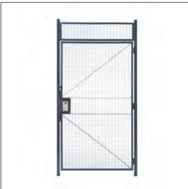
**Hinged Doors** — Hinged Doors swing open to provide access into the cage. Standard Hinged Doors create a 3' or 4'W by 7'-3-1/4"H opening. Other heights are available. The transom panel above the door is sized to match the remaining partition opening. Doors include the transom panel, two door posts and hardware. Each door is hung with three 10 gauge, 4" x 4" tight pin hinges. Doors can be mounted to open from the right or left with inside or outside swing. Order door locks separately.
