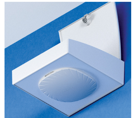
FIGURE 7: Example of a 2 x 2 ceiling mount opened, displaying properly stowed cabling and components for quick and easy authorized access without opening up the ceiling space. The quick-release interchangeable door provides a low-cost method of upgrading to future WAPs.
