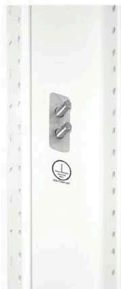
FIGURE 1: Listed Integrated bonding points on painted metal infrastructure eliminate the need for installation professionals to field modify or fabricate bonding connections, while also providing a convenient test point.
