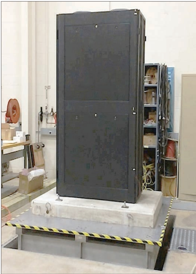
FIGURE 3: A shake-table test ensures that an enclosure will function properly during seismic events. The shake table simulates an earthquake (up to 8.3 on the Richter scale) and shakes the enclosure front-back, side-side and up-down at different levels of intensity.
